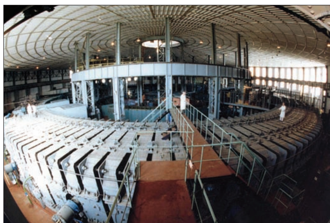
Fig. 2. The 10 GeV Synchrophasotron started up in 1957 as the world's highest-energy accelerator, and is still operational today.
