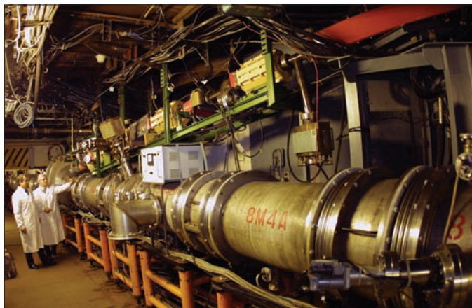
Fig. 4. JINR's Nuclotron – the superconducting synchrotron accelerates nuclei and heavy ions up to 6 GeV/n.
