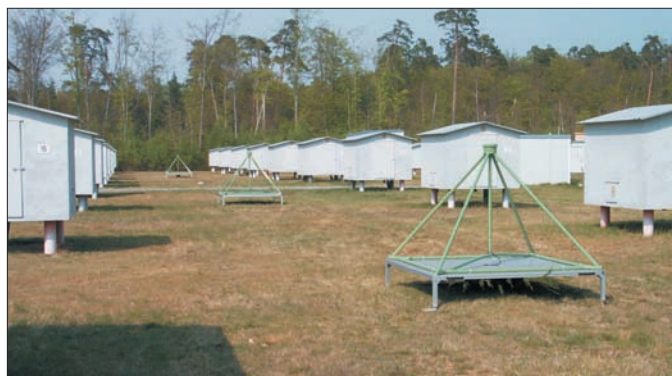
Fig. 3. Three of the LOPES radio antennas between KASCADE particle detectors (the white huts).
