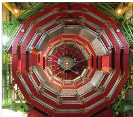
Left: the CMS barrel seen from its +z end in the surface building at Cessy. Two out of five wheels of the barrel are already equipped with muon chambers. Right: a snapshot of the online display showing a cosmic muon (white points) through the complete sector.
